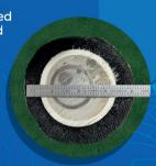
Cutaway of a deep-drilled braced monument leg showing 1/2" rebar, 1-1/4" stainless steel pipe, grout, and foam-wrapped PVC.
